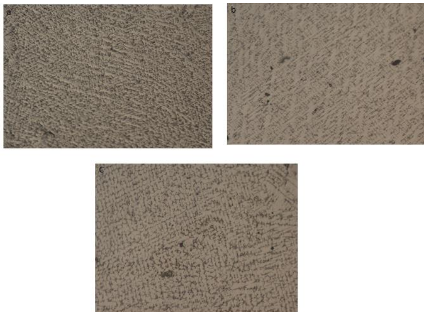
Figure 1 - Optical Microscopic Image of Stellite 6 Alloy Surface on Inconel 718 in Disparate Currents a. 200 Amp, b. 250 Amp, c. 290 Amp (*200)
