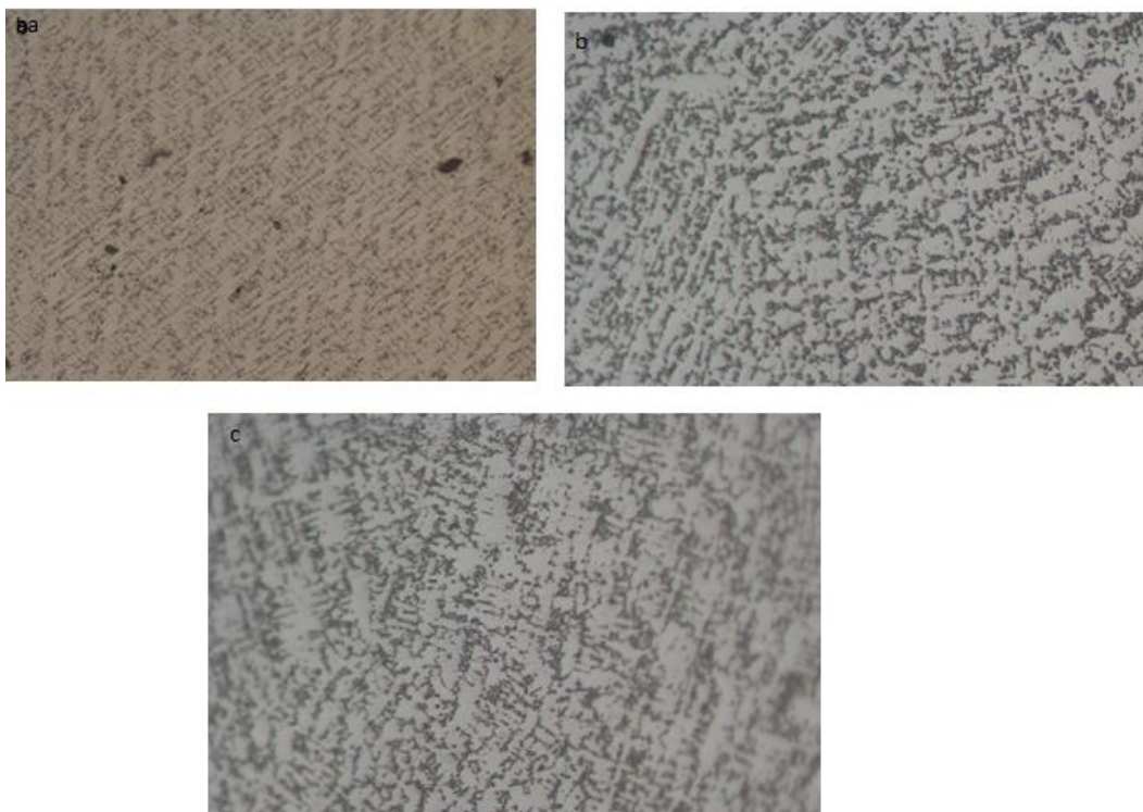
Figure 2 - Optical Microscopic Image of Stellite 6 in Disparate Layers a. Single-Layer Coating, b. Double-Layer Coating, c. Triple-Layer Coating (*400)
