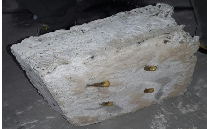
Fig. 2 - UPVT Tested Specimen
