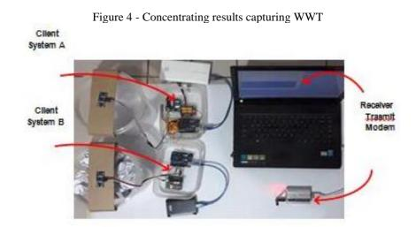
Fig 5 shows the prototype of client method. The client uses the ultrasonic senor located above the model structure of the waste. The radar was linked to the Arduino small controller. Information was processed through the small controller which was send to the global system for mobile communication to the waste transport server.
