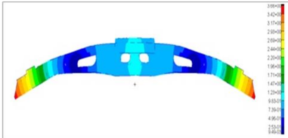
Fig. 11(b) - Mode Shape of Modified Design 218 Hz
