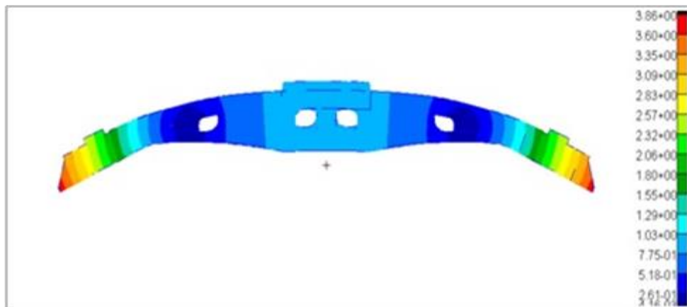
Fig. 11(a) - Mode Shape of Original Design 239 Hz
