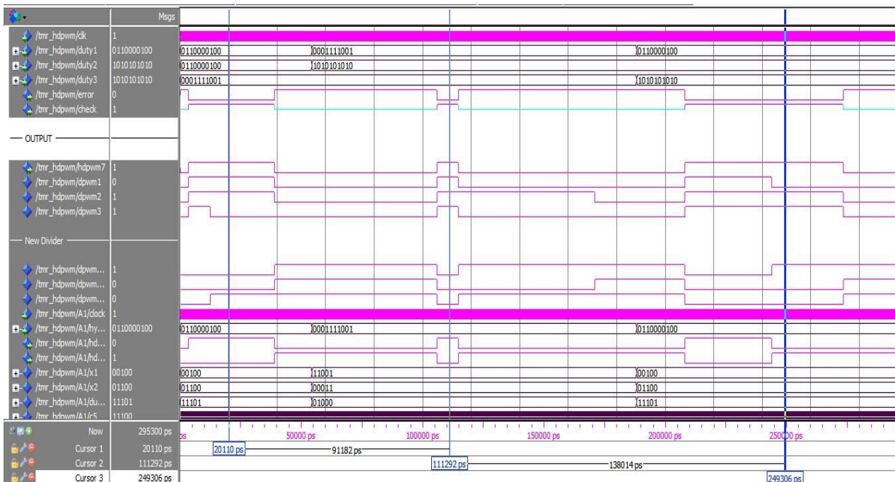
Fig. 7 - Simulation of the Proposed TMR based Hybrid Digital Pulse Modulation
