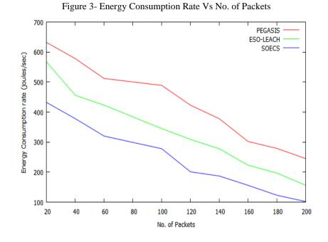
Figure 3 shows the energy consumption rate while varying the number of packets from 20 to 200. The proposed scheme achieves less energy consumption than existing schemes due to the energy estimation of cluster head and non-cluster head.
