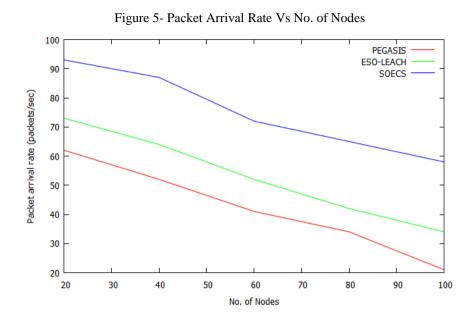
Figure 5 illustrates the performance of SOECS in terms of packet arrival rate. The number of nodes is varied as 10, 20... 100. Due to the deployment of TDMA schedule, packet arrival rate of SOECS is higher than existing schemes.
