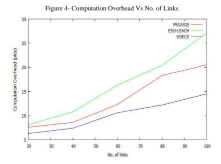
Figure 4 shows the illustration of computation overhead while varying number of links from 20 to 100. From the results, it is seen that SOECS achieves less overhead than ESO-LEACH and PEGASIS.
