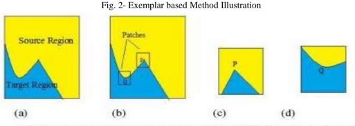
Confidence Term (a) Image to be inpainted; (b) Patches centred around P and Q; (c) Patch with maximum confidence value; (d) Patch with low confidence value.
