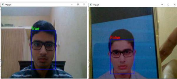
Figure 8- (A) Output for Face Spoofing Detection when an Actual Person is in Front of the Webcam. (B) Output for Face Spoofing Detection when a Photo of a Person is shown in Front of the Webcam
