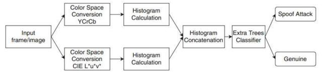
Figure 3- A flow Diagram Describing the various Steps involved in the Process of Face Spoofing Detection
