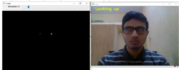
Figure 6- Output for Eye Tracking when the Eyes are looking Upwards and Threshold Value is Set to 27
