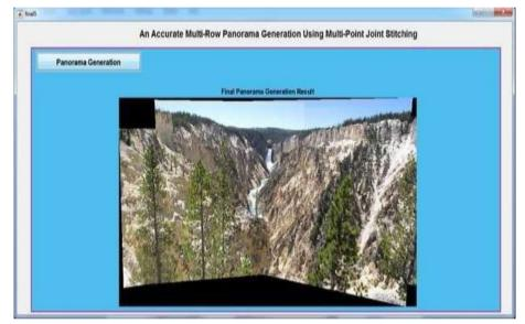
By using the SURF feature based algorithm multiple rows or multiple columns can be stitched at a time so that more accurate multirow panorama can be generated.
