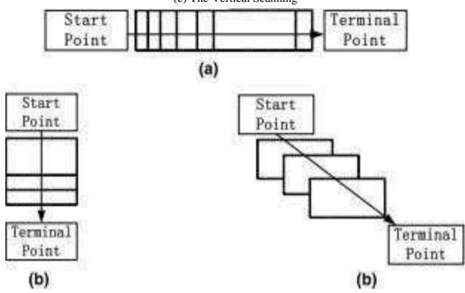
Fig. 1 - Limited Coverage Illustration in 1D Scanning. (a) The Horizontal Scanning. (b) The Oblique Scanning. (c) The Vertical Scanning
